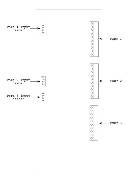
Figure 1 - Port extender board
